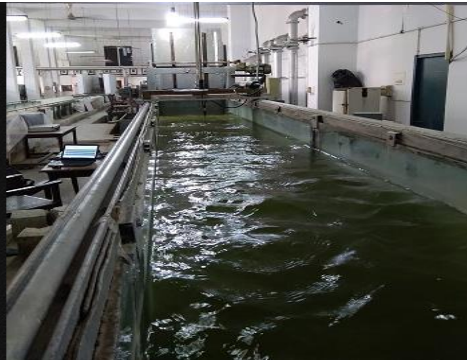
Fig. 6 : (a) Turbulence from mixing of smokes (b) Turbulence in a flume downstream of sluicagate and surface waves due to instability of flow , (hydraulics lab , IIT Roorkee). (c) Turbulence from breaking surface waves in Sunkoshi river along BP Highway
