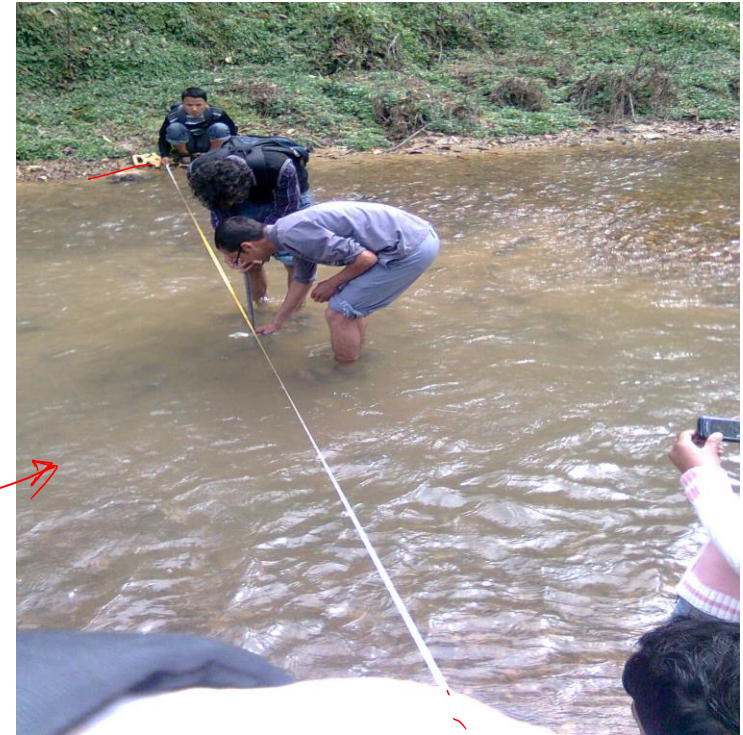
Fig.13 & 14: Typical velocity profile in a channel and photographs 14 shows current meter used for velocity measurement in a stream, Panauti, Nepal
